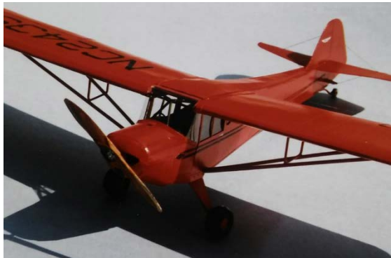
Figure 13. PMI-201 Taylorcraft Model B, Another view of the re-painted model, of potential interest, the designer (Robert Kaelin) recommended that the cabane struts (those that brace the wing roots with the fuselage and are visible as a black inverted "V" immediately behind the clear windscreen) should be fashioned from dry spaghetti noodles. This worked surprisingly well, the noodles are easy to sand, paint and glue, 1/24 Scale, 18" wingspan, four 8.5" x 11" sheets (design 1990: Robert Kaelin, constructed 1996: Matt Vance)
